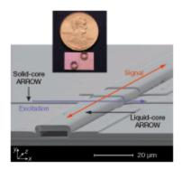
Two antiresonant reflecting optical waveguides (ARROWs), one solid and the other liquid-filled, cross on a silicon platform. The solid waveguide carries the pump light, while the other bears the analyte. The entire platform, including two ring-shaped fluid reservoirs, is smaller than a penny (inset).
