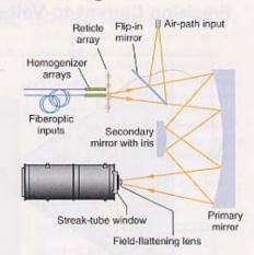
Input optics for the ROSS camera are based on an Offner triplet system. An air path for signals from external sources can be selected with a flip-in mirror, or the homogenizer arrays for fiberoptic signals and internal calibration sources can be used.
